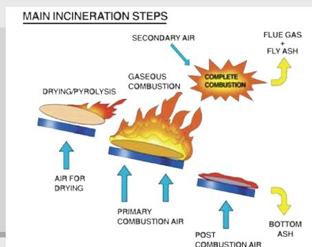
*The main steps in the incineration process are pictured here in a diagram based on a similar model used by Professor Buekens of the VUB University of Brussels. Obviously modern incinerators as used in Western-Europe have to meet the highest EU environmental and health and safety standards in terms of emission controls and energy efficiency.*
